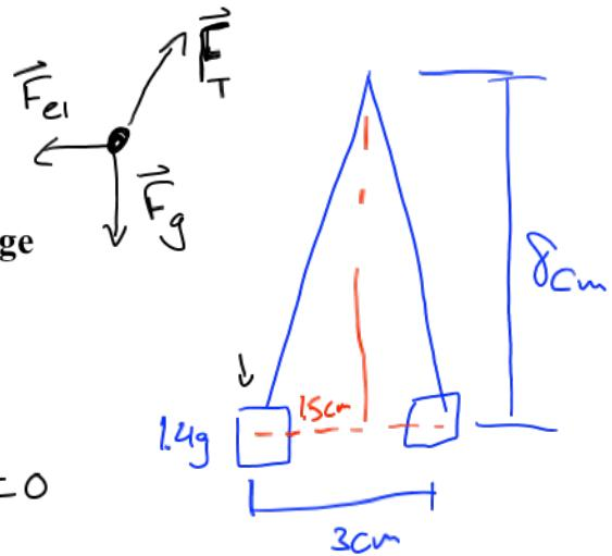
$$\left. \begin{array}{l} 0.184 F_T = \frac{1}{4\pi\epsilon_0} \frac{Q^2}{r^2} \\ 0.983 F_T = mg \end{array} \right\} \begin{array}{l} 2 \text{ eqn} \\ 2 \text{ unknowns} \end{array}$$
